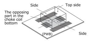
④ This power choke coil is different from the ferrite core-type that installs general concentration GAP. It has the leakage magnetic bunch distribution of the choke coil to the vertical direction. Please be cautious when using parts and circuit compositions which are easily affected by the leakage flux.
