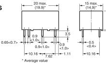
Dimensions in pointed brackets < > are for the Relay mounted to Socket (-P6C).
