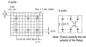
**Fully Sealed Model Single Latching Models** (Straight PCB) G6CU--114P (-FD) -US
