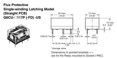
Tolerance: ±0.1 (Bottom View) 1-pole 2 54 Four, 1.1-dia. holes 1-pole S: Set coil R: Reset coil (1.1)
